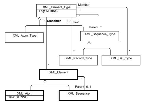
Figure 9. Simplified meta-model of XML-schemas
