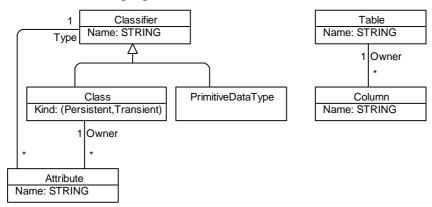
Figure 1. Fragments of UML and RDBMS meta-models
