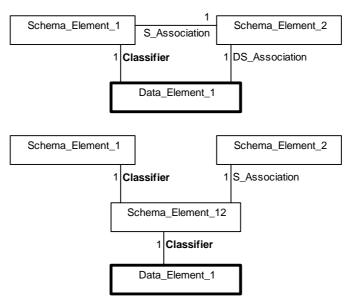
Figure 8. Representing a data-schema association in a schema
