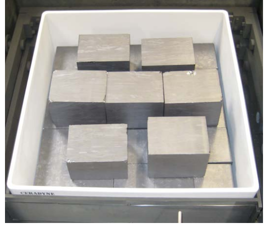
Figure 1.3: Crucible with grown polycrystalline silicon, cut in blocks
