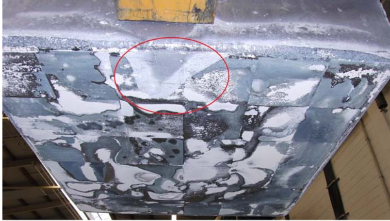
Figure 8.5: Wash-outs in the final silicon block (red circle). Bottom of the block is shown. 6 \times 6 seed crystals were used. Courtesy of ALD Vacuum Technologies GmbH
