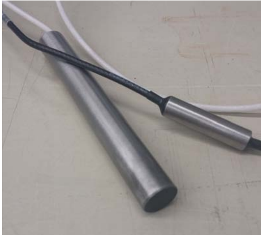
Figure 6.7: 10 mm high-temperature ultrasonic probe from Signal Processing SA
