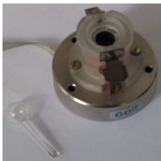
Figure 1. Design of the capillary electrodeless light source - lamp together with HF generator.
