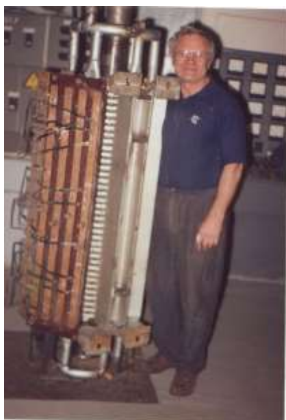
Fig. 1.4. Cylindrical induction electromagnetic pump ( p = 5 bars, q = 10 l/s)
