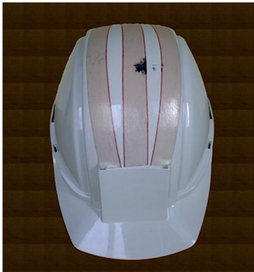
Fig. 2.16. A safety helmet with indication layer strips glued on
