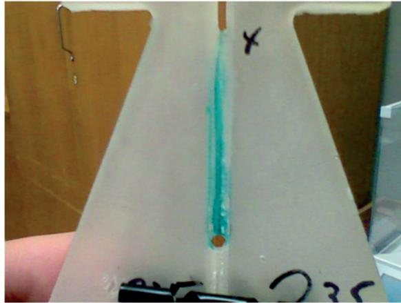
Fig. 3.6. Epoxy TDCB specimen with a crack filled by green dyed alcohol
