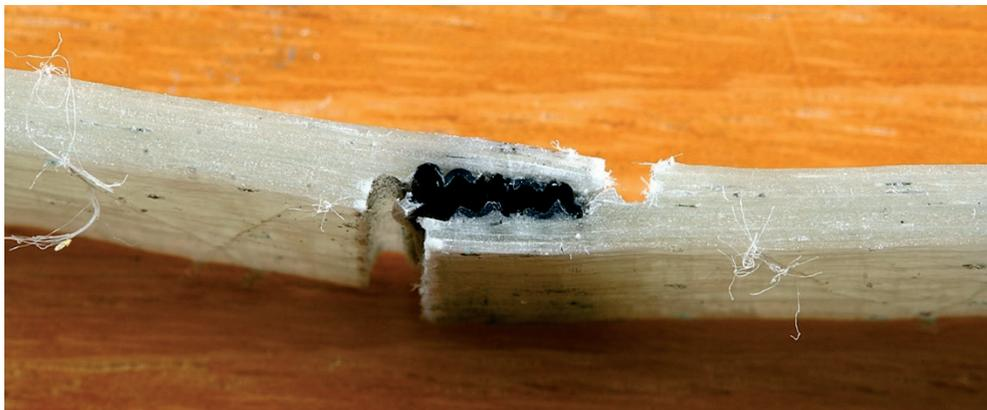
Fig. 3.22. Shear fracture of the damaged D-specimens: the crack propagates through the micro-tubes
