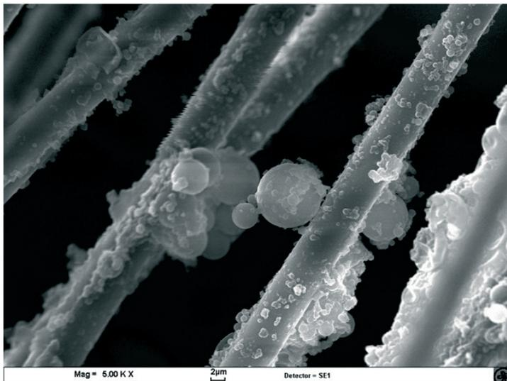
Fig. 2.10. SEM photo of fabric fibres with Microcapsules 500 black copy and Colour developer particles of the developer
