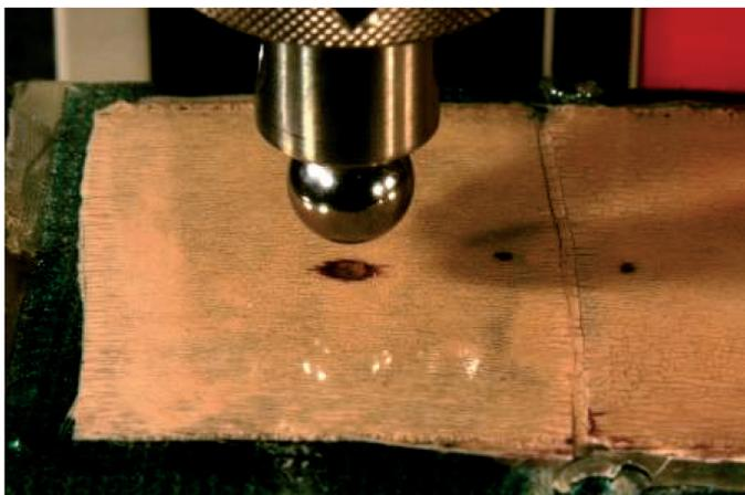
Fig. 2.15. A specimen of the load-bearing composite with indication layer and thin epoxy coating after indentation
