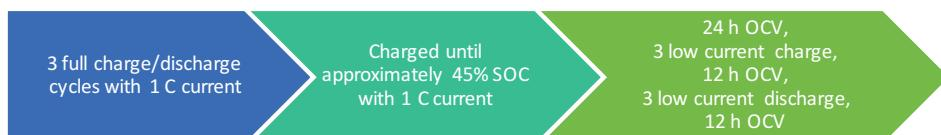
Figure 5.7. Experimental procedure for a single voltage hysteresis measurement
