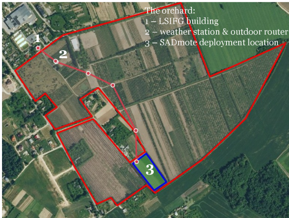
Figure 4.5: The structure and location of SAD WSN in 2011. The points in the middle mark repeater and base station locations
