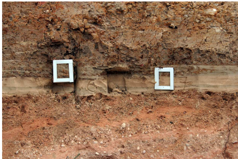
Figure 3.9. The sandy shear zone and samples Nos. ZP6 and ZP7 at a base of the upper till at the Ziemupe site. The height of sampling box is 7 cm. See Fig. 3.3 for location of the sampling site.
