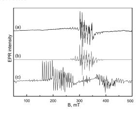
Fig. 6. EPR spectrum of the Mn-doped YAP ceramics sample (the same as in [9]) measured at the temperature 77 K and microwave frequency of 9.14 GHz. (a) Experimental spectrum, (b) and (c) are simulated spectra with the  $\rm Mn^{2+}$  (b) and  $\rm Mn^{4+}$  (c) EPR parameters from [14].
