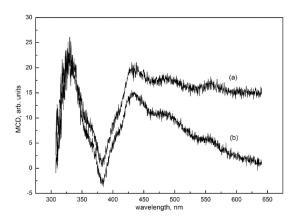
Fig. 4. MCD spectrum of the Mn-doped glass-ceramics, measured at B=2 T and temperature 1.5 K (a) and 4.2 K (b).
