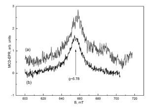
Fig. 2. MCD-EPR spectrum of the Er-doped glass-ceramics sample, measured at two different MCD bands — 377 nm (a) and 521 nm (b) at T=1.5 K and at the microwave frequency 62 GHz. The magnetic field dependent background has been subtracted. The resonance at  $g\approx 6.78$  corresponds to the cubic Er<sup>3+</sup> in CaF<sub>2</sub> crystallites.
