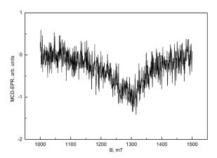
Fig. 5. MCD-EPR spectrum of the Mn-doped glass-ceramics sample, measured at temperature 1.5 K in the 430 nm MCD band, with the microwave frequency of 35 GHz. The magnetic field dependent background is subtracted.
