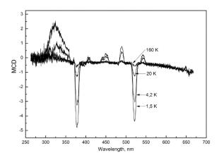
Fig. 1. Temperature dependence of the MCD spectrum of the Er-doped glass-ceramics sample measured at B=1 T. So-called paramagnetic behaviour for all the MCD bands has been observed.
