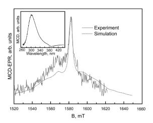
Fig. 3. MCD-EPR spectrum of the  $\mathrm{Gd}^{3+}$ -doped glass ceramics sample measured at the 44.2 GHz microwave frequency. The spectrum could be well simulated with the EPR parameters of the cubic  $\mathrm{Gd}^{3+}$  in the  $\mathrm{CaF}_2$  crystallites (for more details see [8]). Inset shows the corresponding MCD spectrum of the glass-ceramics, measured at T=4.2 K and B=1 T.
