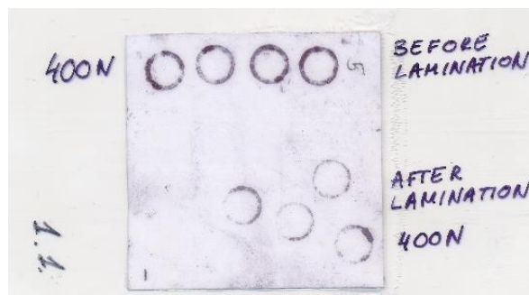
Figure 2.10. Example of the laminated DVIS; the sensitivity of the sample to external load before and after lamination was compared.
