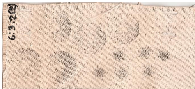
Figure 2.17. Sample after compression test with two types of indenters.
