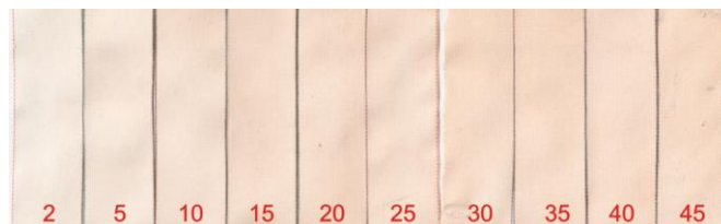
Figure 2.21. Samples of the DVIS after UV irradiation from 2 till 45 min.
