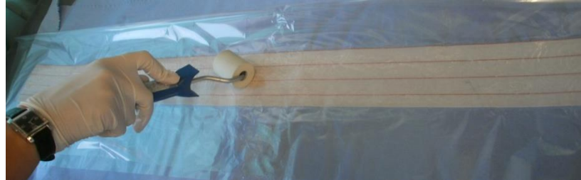
Figure 3.3. Sample aligning and bubble removal.
