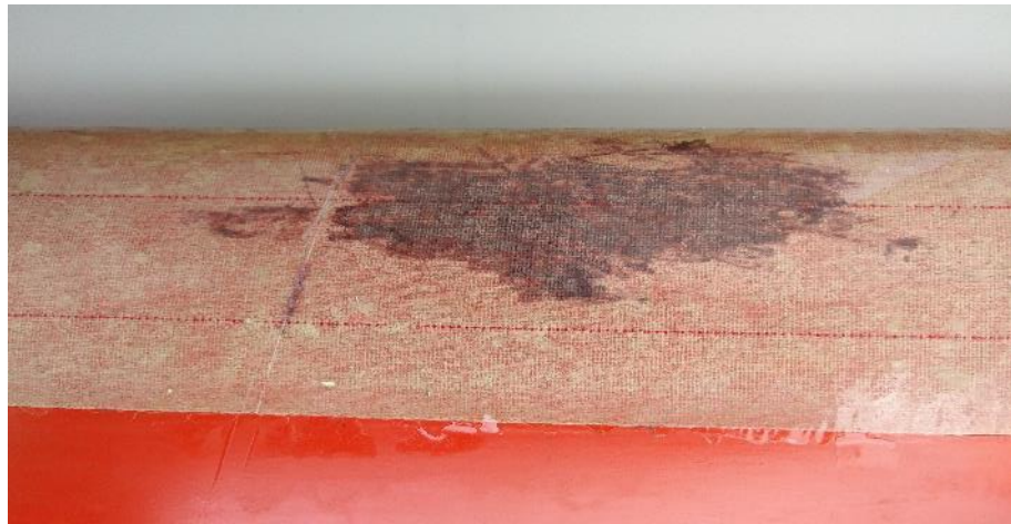
Figure 3.5. Composite wind turbine blade with the DVIS as an external layer; the DVIS as a prepreg is located on the top of the blade (1), using rubber roller it is pressed to the surface (2), blade with a glued DVIS was covered by PET film and left for the curing of the resin (3), wind turbine blades with and without the DVIS (4), place of the applied load is identified with a colour change (5).
