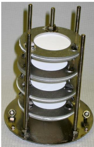
Fig.1.1. Four POCIS mounted on a stainless-steel deployment canister
