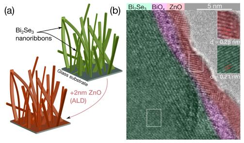
**Figure 1.** (a) Schematic representation of catalyst-free PVD-synthesized free-standing  $Bi_2Se_3$  nanoribbons on glass substrate; (b) false-colored HR-TEM image of a  $Bi_2Se_3$  nanoribbon after encapsulation with a thin layer of ZnO.
