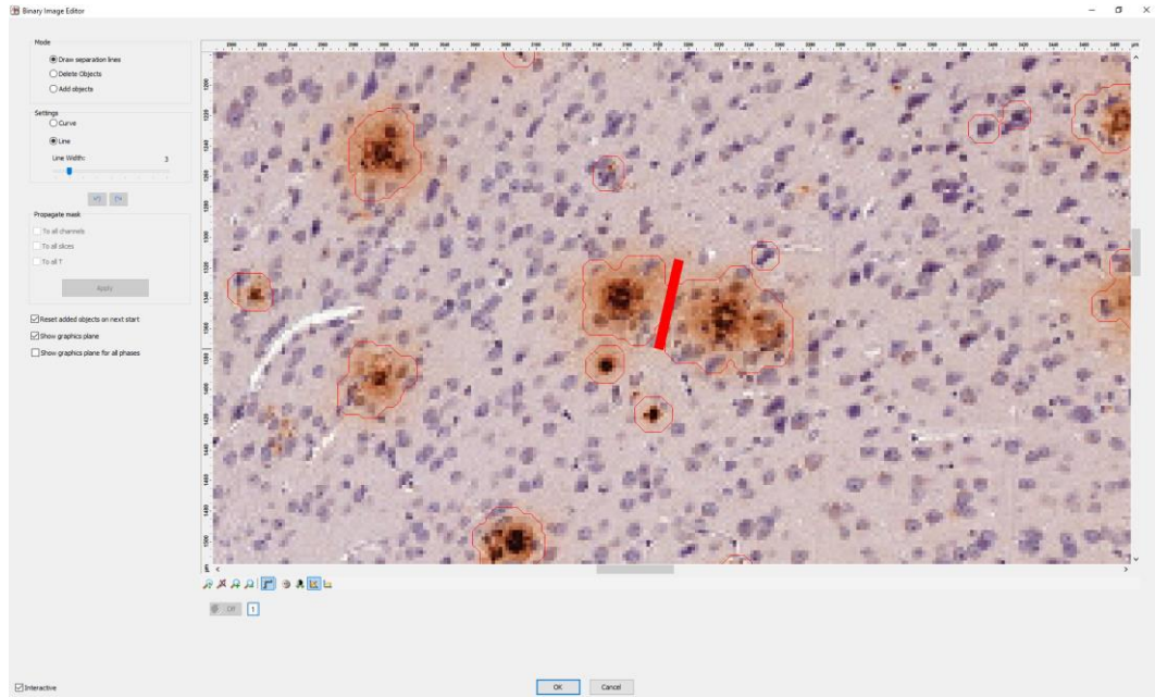
Fig. 9. Separation of plaques: how to separate two plaques that have been detected as one object using the line tool in our custom script in AxioVision.
