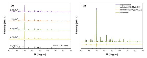
**Figure 1.** (a) XRD patterns of  $Sr_2MgSi_2O_7$  samples doped with 0–3%  $Pr^{3+}$ ; (b) Rietveld refinement data of the 3.0%  $Pr^{3+}$  sample.
