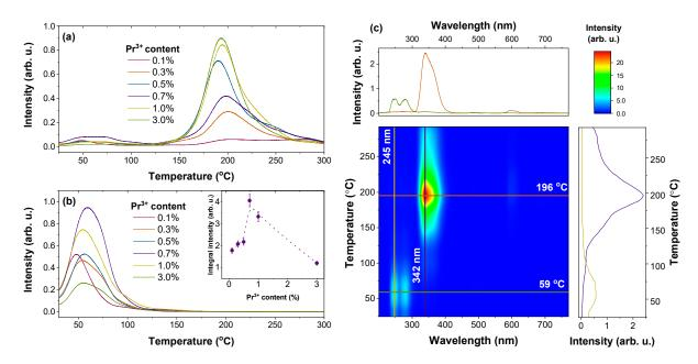
**Figure 4.** TSL glow curves of (a) full emission and (b) filtered UV-C emission of  $Sr_2MgSi_2O_7$  samples doped with 0.1–3.0%  $Pr^{3+}$  after 30 s irradiation with X-rays; inset: integral TSL intensity dependence on  $Pr^{3+}$  concentration; (c) wavelength-resolved TSL contour plot of  $Sr_2MgSi_2O_7$  doped with 0.7%  $Pr^{3+}$ .
