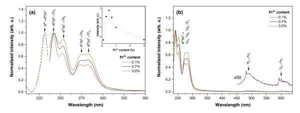
**Figure 2.** (a) PL excitation spectra monitoring 243 nm emission (dashed lines) and PL spectra in the UV range excited with 232 nm (solid lines); inset: integral UV-C emission intensity dependence on  $Pr^{3+}$  content; (b) PL spectra in UV and visible ranges excited with 232 nm of  $Sr_2MgSi_2O_7$  doped with 0.1–3.0%  $Pr^{3+}$ .
