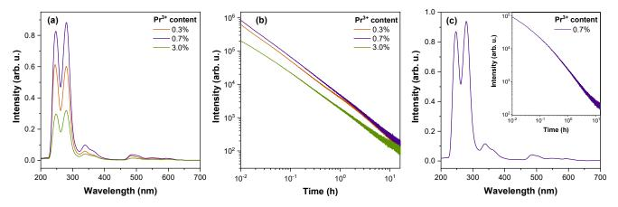
**Figure 3.** (a) Persistent luminescence spectra and (b) UV-C emission decay kinetics of  $Sr_2MgSi_2O_7$  samples doped with 0.3–3.0%  $Pr^{3+}$  after irradiation for 3 min with X-rays at room temperature; (c) persistent luminescence spectrum of the 0.7%  $Pr^{3+}$  sample irradiated for 10 min with 232 nm; inset: UV-C persistent luminescence decay kinetics of the same sample.
