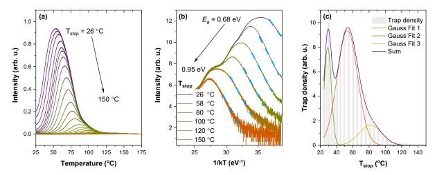
**Figure 5.** (a) TSL glow curves of the 0.7%  $Pr^{3+}$  sample measured after preheating to  $T_{stop}$  from 26 to 150 °C; (b) IRA of selected data obtained from the  $T_{max}$ – $T_{stop}$  experiment; (c) the calculated trap density distribution.
