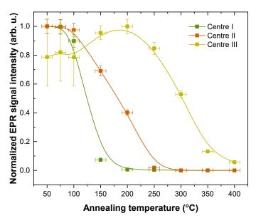
Figure 7. Annealing kinetics of the individual EPR signals.
