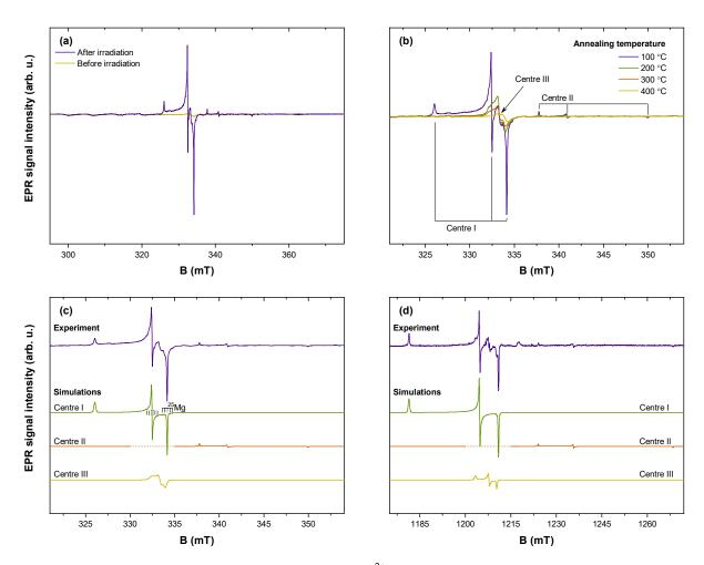
**Figure 6.** EPR analysis of the 0.7% Pr<sup>3+</sup> sample: (a) experimental spectra before and after irradiation with X-rays; (b) spectra evolution with sample annealing temperature; simulations of individual signals contributing to EPR spectra detected at (c) X and (d) Q microwave frequency bands.
