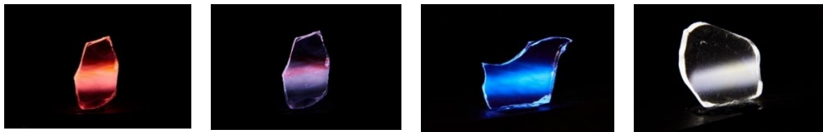
Figure 3.4. Photographs of luminescence in oxyfluoride glasses: a) \text{Eu}^{3+} ions ( \lambda_{\text{ex}}=320 nm); b) \text{Eu}^{3+} and \text{Eu}^{2+} ions ( \lambda_{\text{ex}}=350 nm); \text{Eu}^{2+} ions ( \lambda_{\text{ex}}=350 nm); \text{Tb}^{3+} and \text{Eu}^{3+} ions ( \lambda_{\text{ex}}=350 nm).
