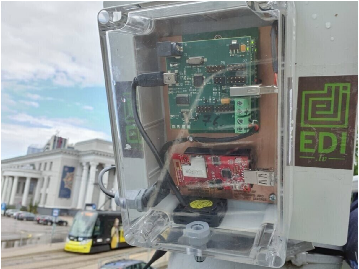
Figure 4.3: EDI TestBed Workstation with modified enclosure
