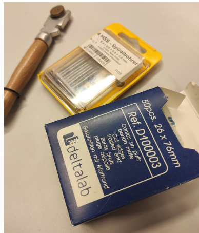
(b) A glass cutter, diamond dust coated jewellery drill bits (in the yellow case) and a box of used microscope glass slides.
