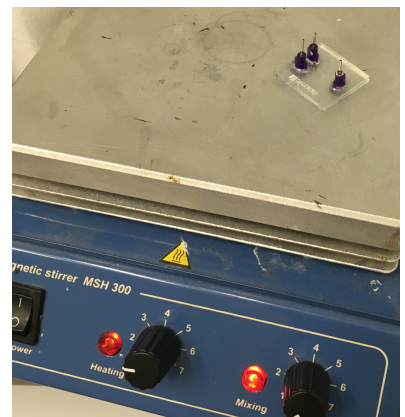
(f) Heating of the microfluidics chip with a hot plate (Biosan MSH-300). This is last step of the preparation.
