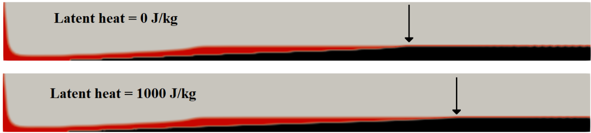
Fig. 3.6.32. Metal casting test case results: black - solid metal, red - liquid metal, grey - air. The black arrows mark the point from which the layer is completely solid.
