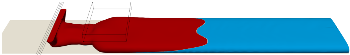
Fig. 5.4.17. Phases at steady state with combined AC and static magnetic field, I = 1 kA, M_0 = 1 T; red - liquid, blue - solid.
