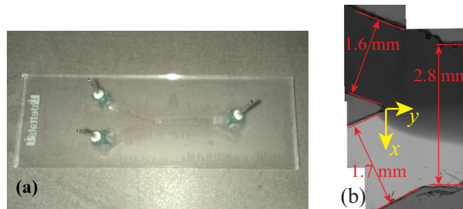
Figure 3.8: Microfluidics flow cell with a Y channel system, fabricated by welding two microscope slides with a patterned Parafilm M® spacer. (a) Image of the actual setup. Microscope slide is 75 mm long. (b) A collage of microscope images of the channel connection point with channel width measures. Yellow arrows mark the definition of coordinate axis with an origin fixed at the tip.
