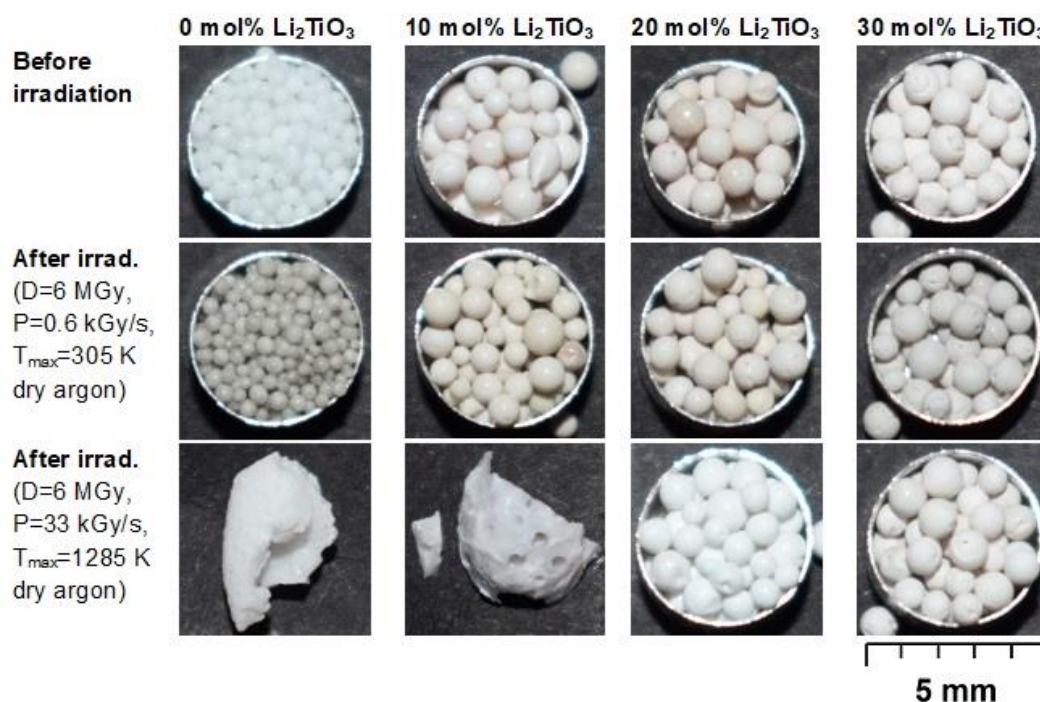
Fig. 3.1 Photos of the Li_4SiO_4 pebbles with various contents of Li_2TiO_3 before and after irradiation with 5 MeV accelerated electrons up to 6 MGy absorbed dose at around 305 K and up to 1285 K in a dry argon atmosphere.
