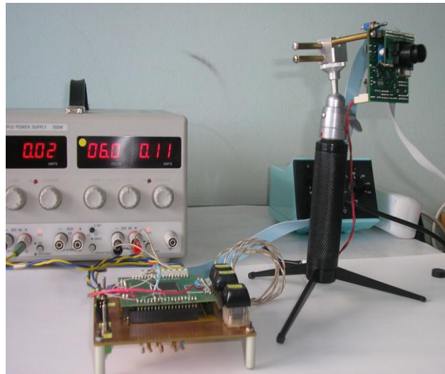
Figure A7.6 The developed asymmetric data capturing device.
