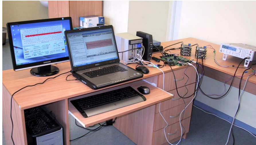
Figure A3.1 Novel multi-channel data acquisition system prototype. The system's front-end part is based on SWC sampling principles, involving data transmission with timing instants.
