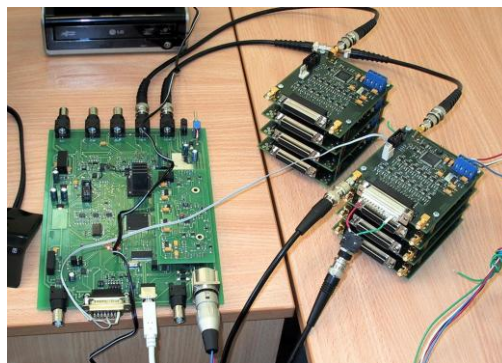
Figure A3.2 Developed multi-channel DAQ system.
