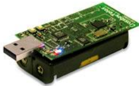
Figure 2.6 Sensor mote TelosB from Crossbow illustrating state-of-the-art in the field wireless sensor networks.
