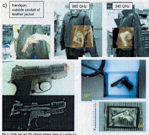
Fig. 3. Visible (top) and TIR reflection (bottom) images of a section of a plastic gun taken at a distance of 1 meter.
