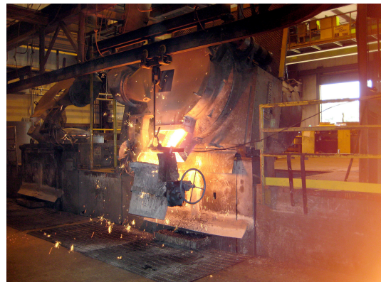
Figure 2.1: A sketch of the typical ICF, where inductor is placed around the crucible, which is filled with the melt and operation of such furnace at “Gartland Foundry”.
