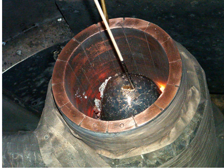
Figure 5.2: Temperature measurements in liquid Aluminium with thermocouple placed in a protective ceramic tube.
