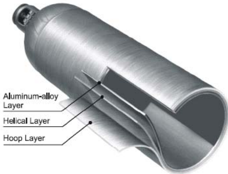
Figure 1.3.1.1: A cylinder with a thin metal liner of steel or aluminium and a fully wound composite over wrap [41]
