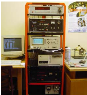
Fig. 4.3. Dielectric spectroscopy set up of frequency and temperature dependencies measurements.
