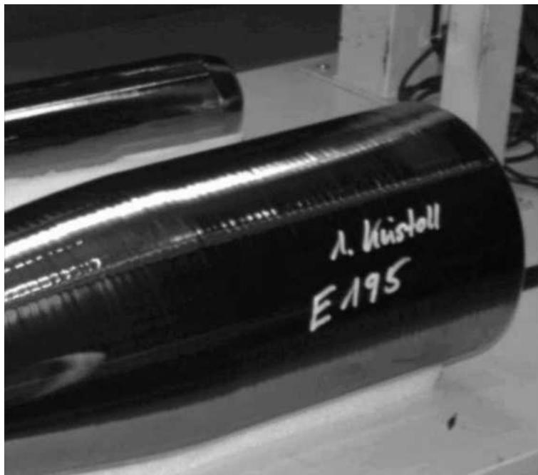
Figure 2.1: The worldwide first dislocation-free 200 mm FZ silicon crystal (courtesy of Siltronic AG).
