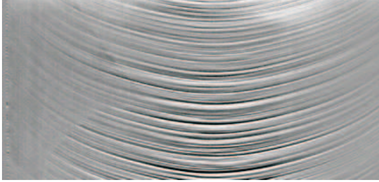
Figure 5.16: The photo-scanning resistivity measurement in the vertical cross-section of an 8 inch FZ crystal (Siltronic AG) has been performed at the Institute of Crystal Growth [88].
