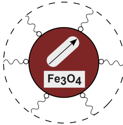
Figure 1.1: Visual representation of a sterically stabilized ferrofluid magnetite particle. The red circle represents the magnetic core made of magnetite. The size of this core is referred to as magnetic size. The dashed line represents the entire colloidal particle - magnetic core together with a layer of surfactant. The size of this particle is referred to as hydrodynamic size
