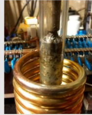
Example of molten and then solidified tin mass in a crystal growth tube suspended above the induction coils
