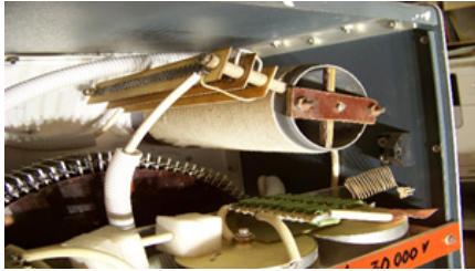
Fig. 8. Dempfer coils with 2 kW composite resistor
