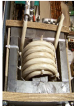
Fig. 12. A part of HV rectifier with cooler platelets
