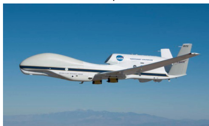
NASA's remotely piloted "Global Hawk" aircraft NASA's Goddard Space Flight Center (flight duration 30 hours, altitude up to 18 000 km)
