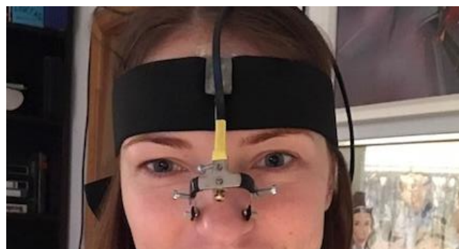
Figure 2.8 Strain gauge unit fixation to the metal bridge and headband
