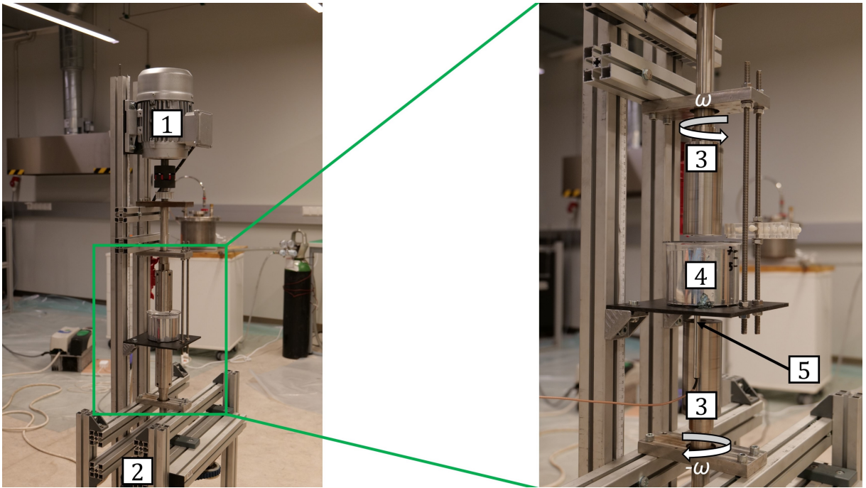
Figure 6.1: Experimental rig for two magnet shear flow: 1 - electric motor driving upper magnet; 2 - lower magnet motor; 3 - permanent magnets ( D=50 mm, H=100 mm, f=10 Hz), magnetization is radial (see blue arrows); 4 - GaInSn container ( D=100 mm, H=70 mm); 5 - UDV probe measuring axial velocity
