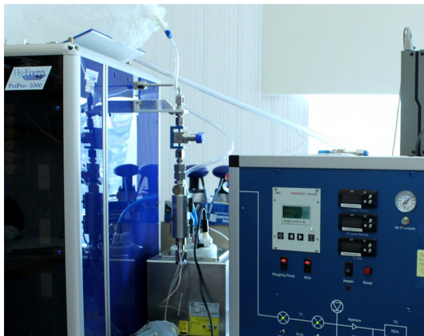
Fig. 2.2. Masspectrometer RGAPro-100 connected with bioreactor and microsensors in water bath (photo Dimanta, 2014).
