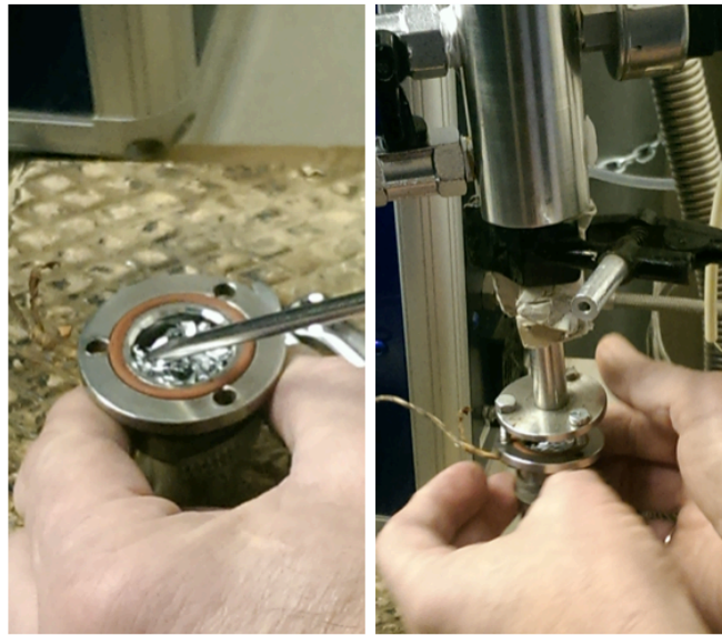
Fig. 2.3. Activation of metal hydride powder in cylindrical stainless steel hydrogen adsorption/desorption reactor (photo Dimanta, 2014).
