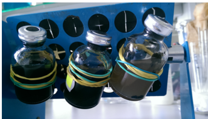
Fig. 2.4. Serum bottles rotation with microorganisms, medium and metal hydride powder (photo Dimanta, 2014).
