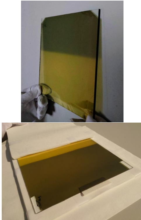
Figure 6-2 | Natural photochromic efficiency of YHO. A 200 mm 2 photochromic YHO sample was exposed to sunlight for 15 minutes, visually displaying its transparent and Photodarkened states.
