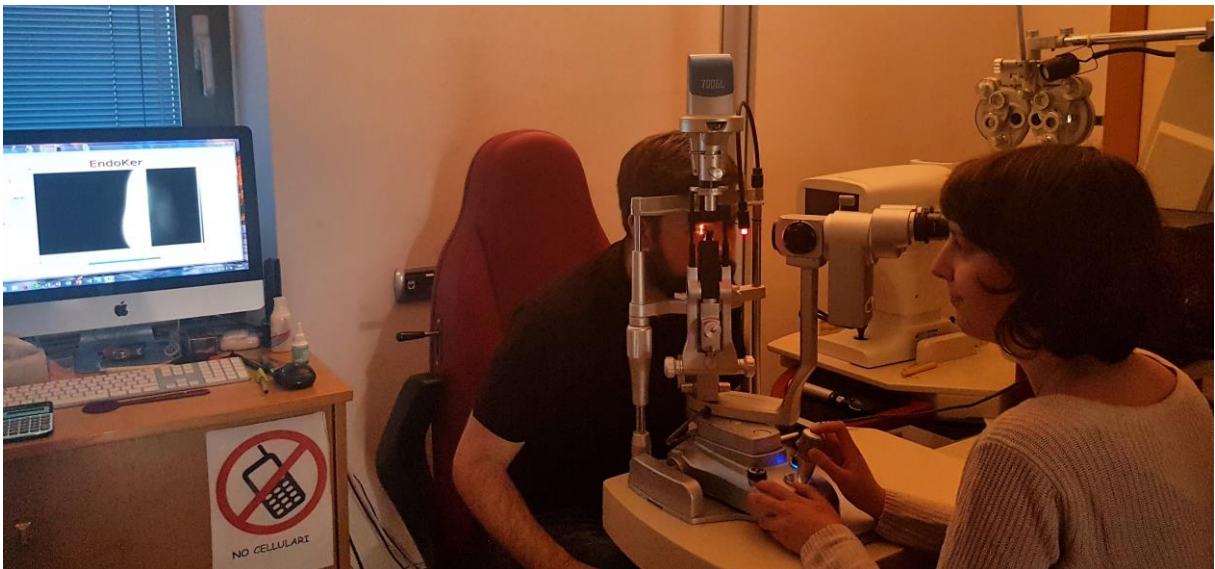
Fig.2.1. Taking pictures with Takagi 700GL slit lamp with EndoKer external elaboration system.
