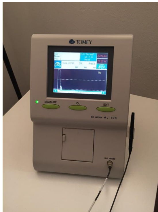
Fig. 2.2. Ultrasound SCAN Biometer AL 100 by TOMEY CORPORATION.
