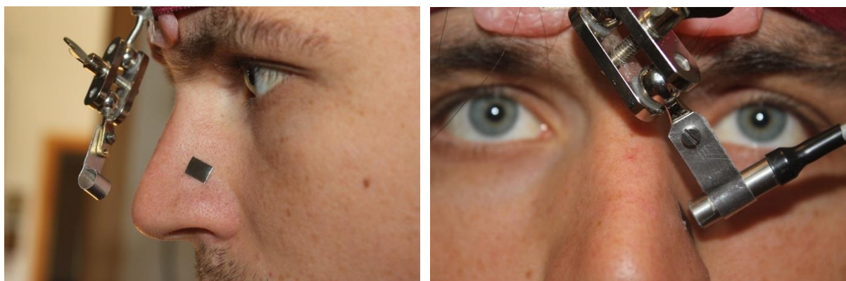
Figure 2.3 - Left: Lateral view of the metal plate taped to the external nose; Right: Frontal view of the inductive sensor by Baumer in its retainer, positioned closely to the metal plate
