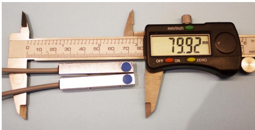
Figure 2.5 - Inductive sensors by Contrinex; blue circles mark the sensing area
