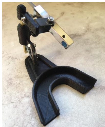
Figure 2.7 – Setup of the inductive sensor by Contrinex used in advanced laboratory testing showing the chrome-colored sensor with the blue sensing area on a 3D-printed mounting apparatus and bite plate
