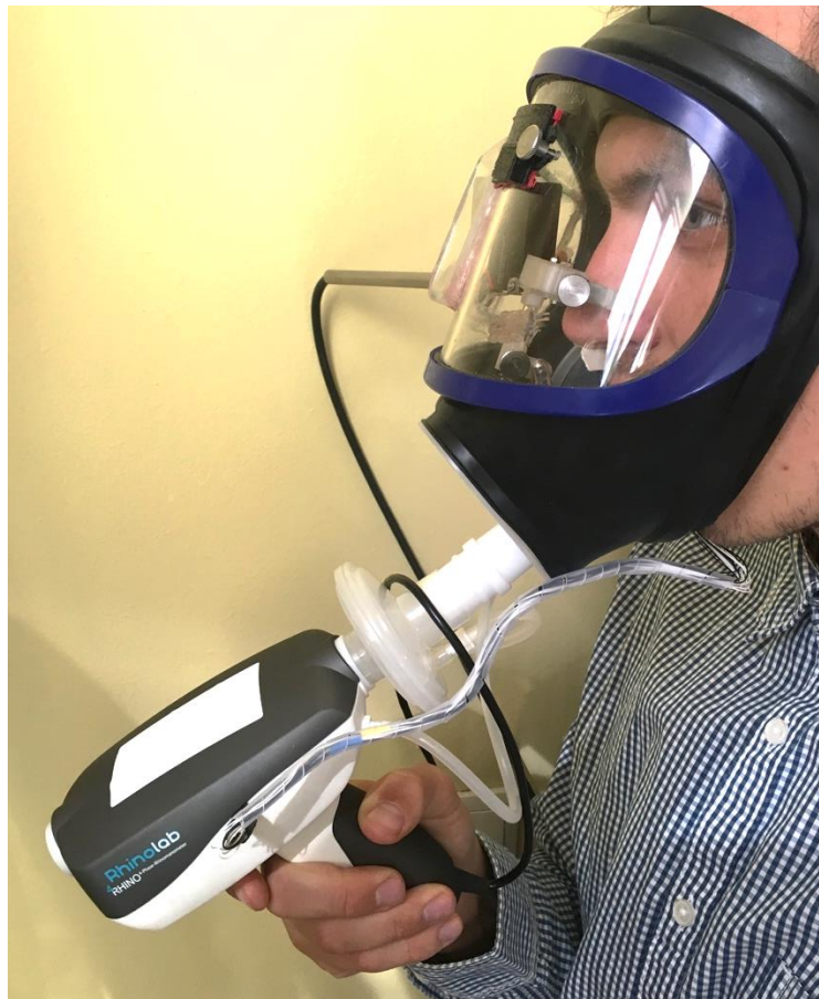
Figure 2.11 – Image showing the setup for comparison used in participant testing with the strain gauge placed on the lateral external nasal wall, the laser directed at it on the right side of the nose and the 4-phase rhinomanometer recording
