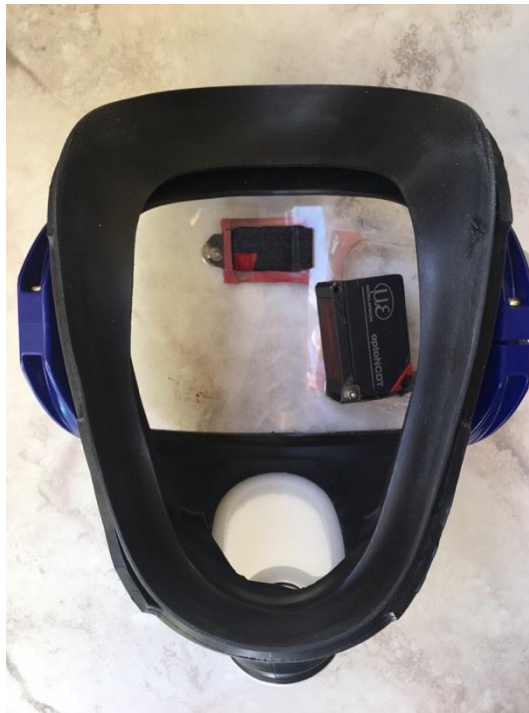
Figure 2.9 – View of the interior of the facemask used in participant-testing with the optical sensor by MicroEpsilon below the visor on the right
