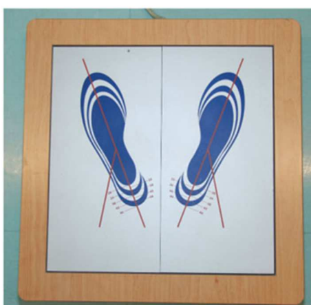
Figure 2.1 Stabilometric computerized platform, Postural Health Station (DL Medica SpA, Milano, Italy) demonstrating the position of feet during the measurement (Baldini, et al., 2013).
