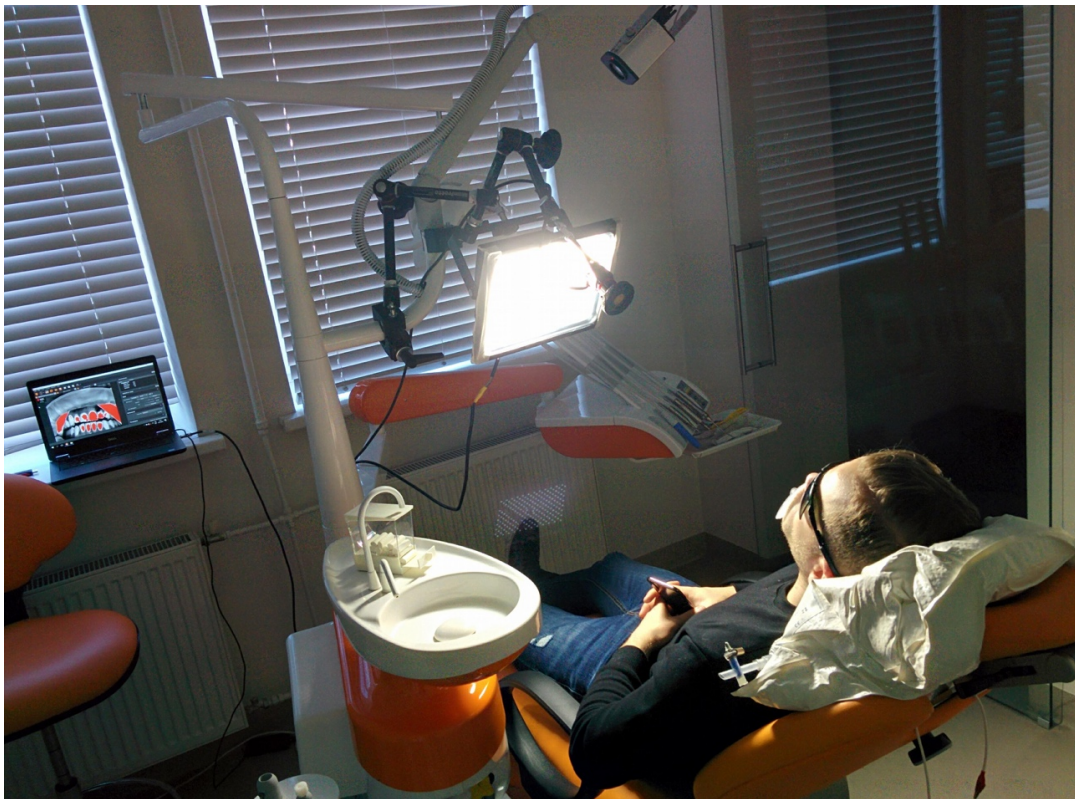
Figure 10 shows how the subject is seated in the dental chair with the head fixed in a vacuum support pillow and the iPPG setup.
