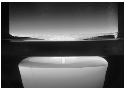
f0050 FIGURE 6.9 Formation of a “nose” that cannot be molten inductively and can lead to a process crash.
