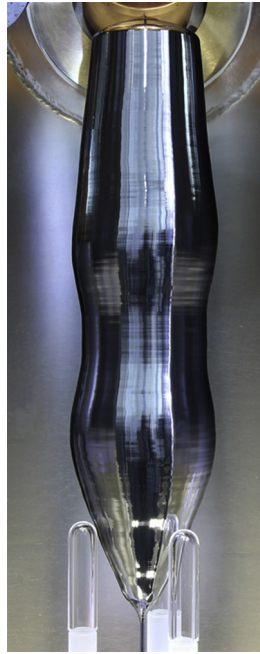
f0065 FIGURE 6.12 Image of the grown Avogadro crystal using regulation. The image was taken by Turschner at the Leibniz Institute for Crystal Growth (IKZ).
