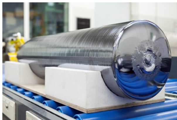
f0015 FIGURE 6.2 A silicon monocrystal with 200-mm diameter grown at Siltronic AG using the floating zone process. Photo: Siltronic AG.
