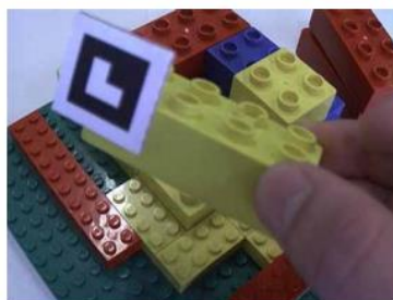
(a) Lego brick and hand are rendered opaquely. An AR Toolkit marker is attached to the brick so that its position and pose can be tracked.
